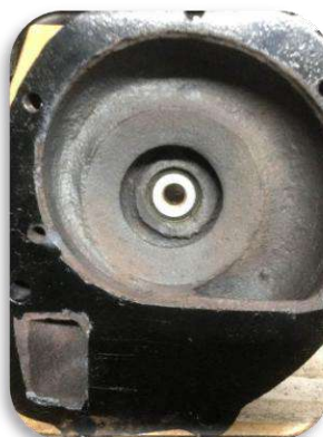
Above: The carbon seal was machined out suit the ceramic insert and a new bronze bush installed for the impellor spindle.
