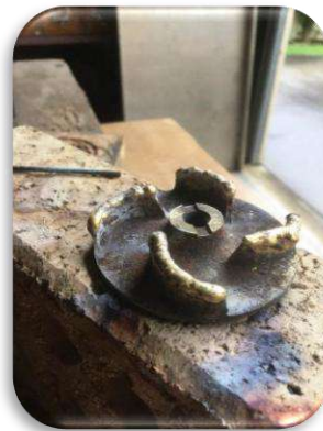
Above: The impellor being badly worn was built up about 5 mm with bronze.
